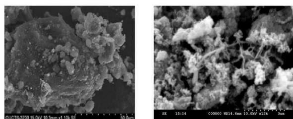
Pd10/CB catalyst before test Pd10/CB catalyst after test
