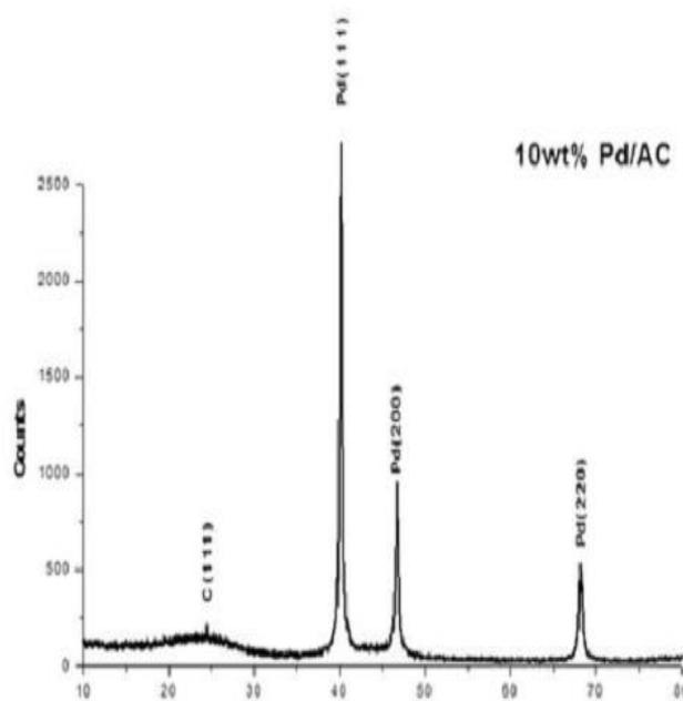
Fig. 5 - XRD Analysis of Pd10/AC
