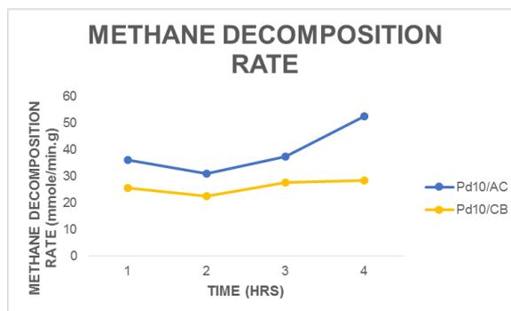
Fig. 4 - Methane decomposition rate (mmole/min.g) in Pd10/AC and Pd10/CB
