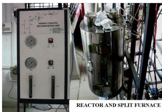
Fig. 1 - Thermo catalytic decomposition reactor setup
