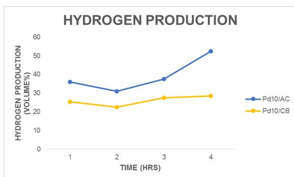
Fig. 2 - Hydrogen production (Volume %) in Pd10/AC and Pd10/CB
