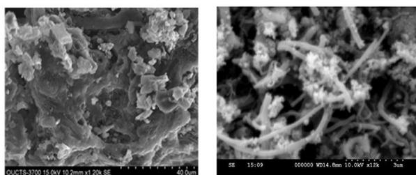
Pd10/AC catalyst before test Pd10/AC catalyst after test
