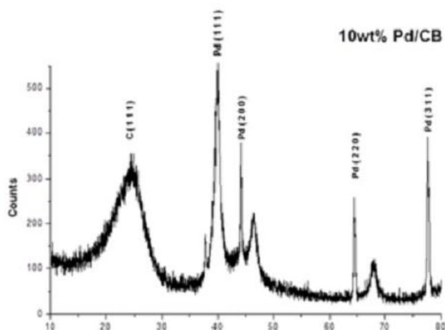
Fig. 6 - XRD analysis of Pd10/CB
