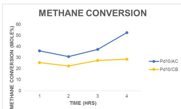
Fig. 3 - Methane conversion (mole %) in Pd10/AC and Pd10/CB
